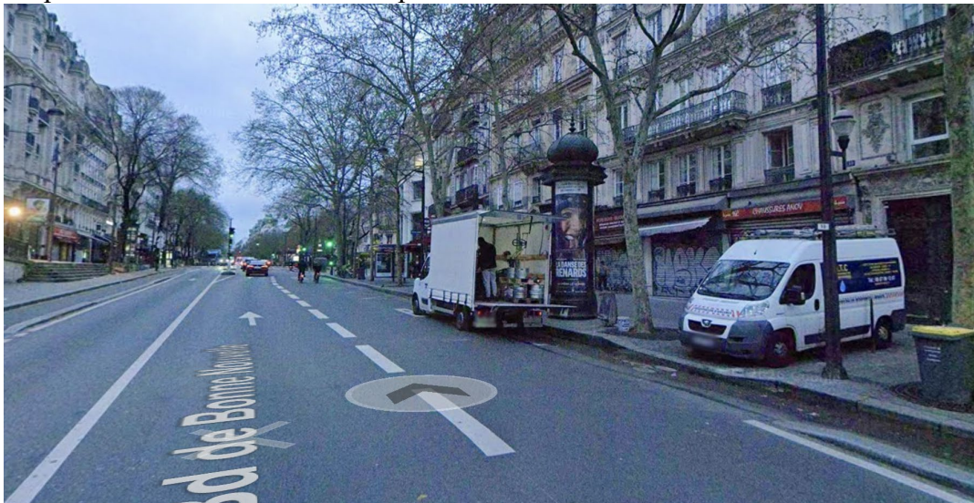
5 Bd de Bonne Nouvelle, 40 ft curb-to-curb. Bike lanes separated by low mountable curb, allowing a delivery truck to stop in one of them.
