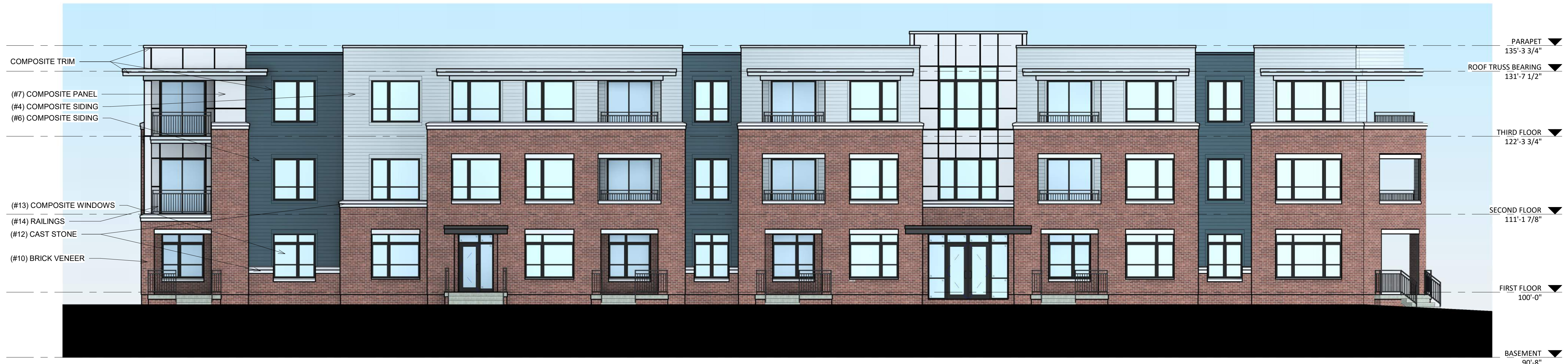
1 COLORED ELEVATION - BLDG 3 A202 1/8" = 1'-0"
