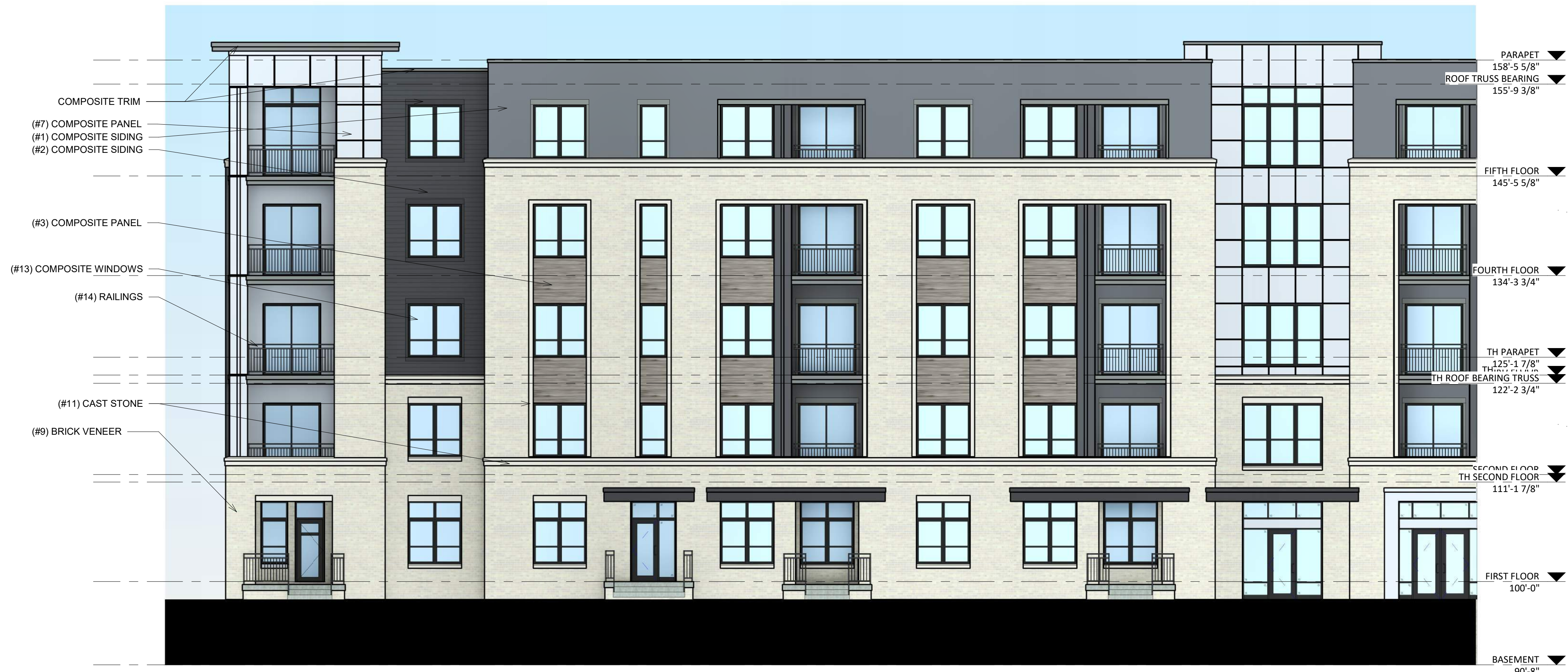
1 COLORED ELEVATION - BLDG 1 1.0 A202 1/8" = 1'-0"
