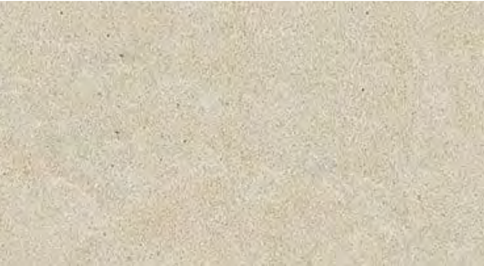
CAST STONE (BASE WAINSCOT AND WINDOW SILLS)
