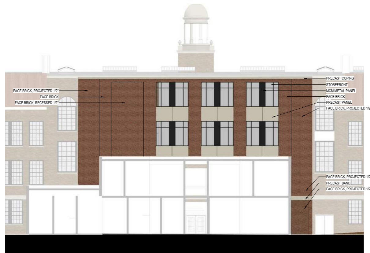
A3 ELEVATOR ADDITION - WEST - UDC 1/8" = 1'-0"
