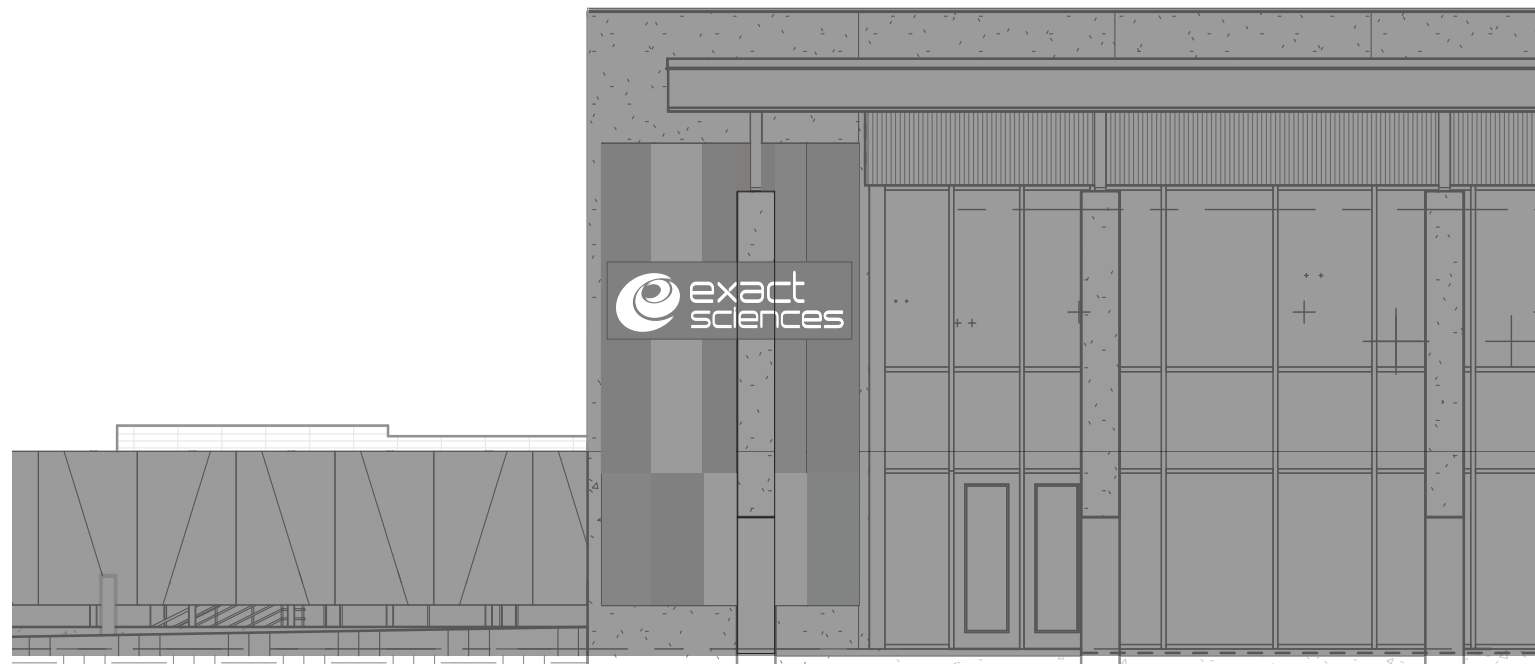
SIGN TYPE F - BUILDING FACADE ID - ENTRANCE FROM FORWARD DRIVE (HALO LIT)
