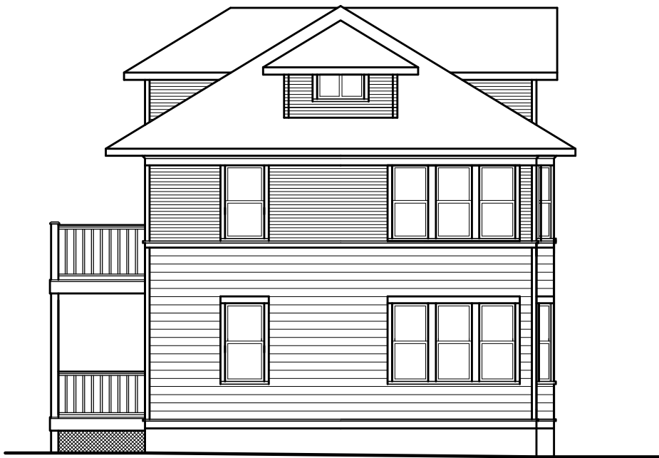
NORTH ELEVATION SCALE 1/4" = 1'-0"
