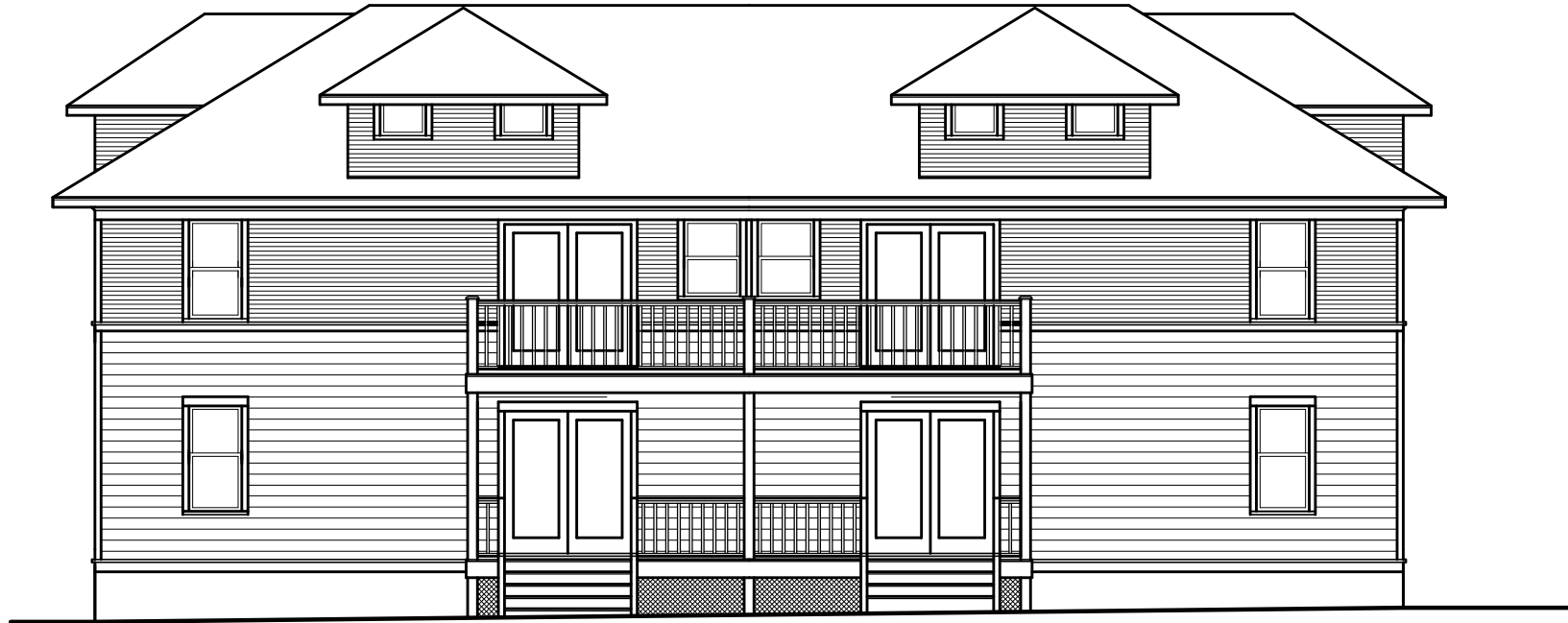
EAST ELEVATION SCALE 1/4" = 1'-0"
