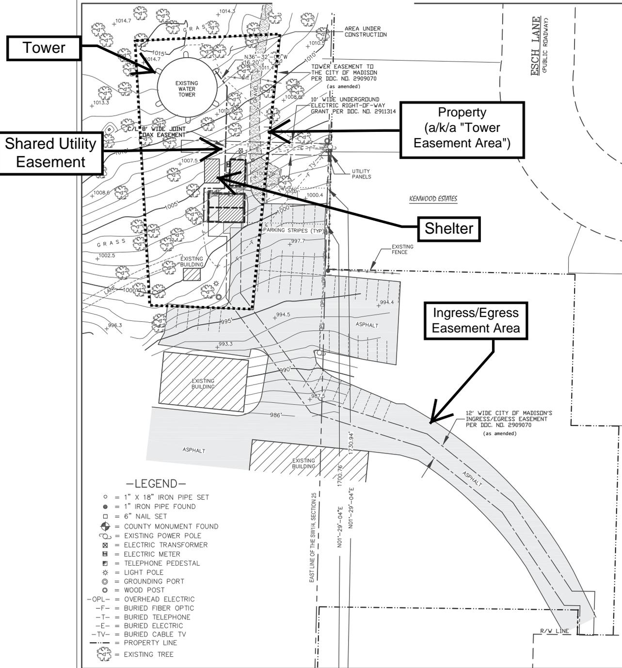
BEARINGS REFERENCED TO THE DANE COUNTY COORDINATE SYSTEM AND THE EAST LINE OF THE SW1/4 SECTION 25, T8N, R9E, WHICH BEARS N01°29'04"E
