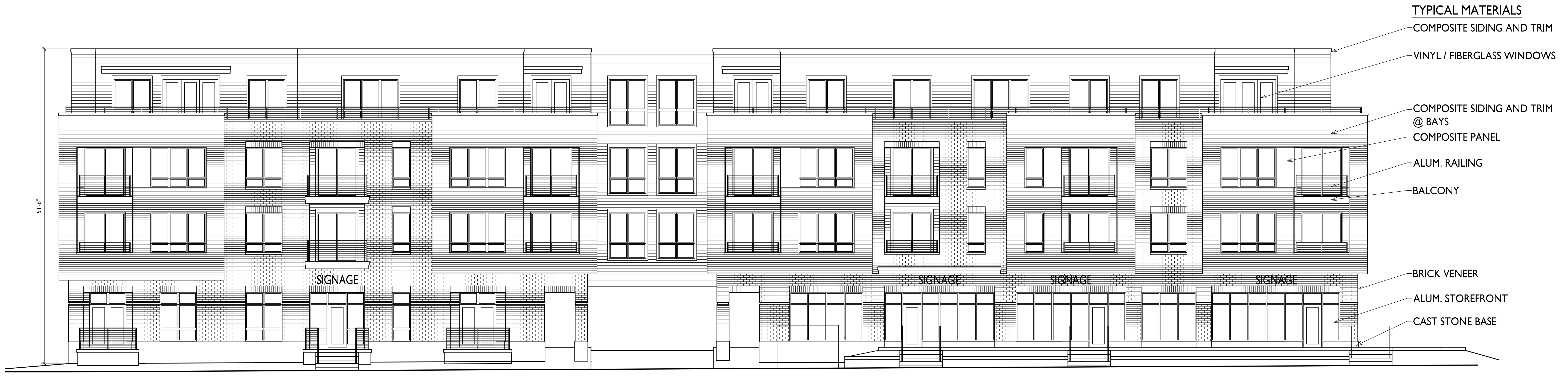
1 A-2.1 1/8" = 1'-0" NORTH ELEVATION ALONG UNIVERSITY AVENUE
