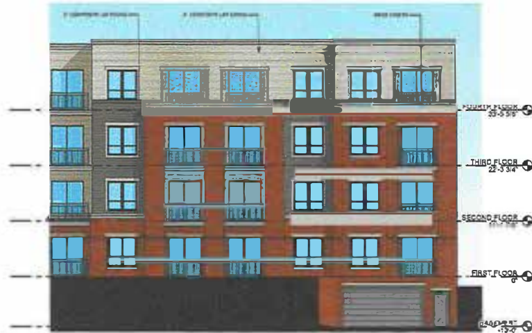
2 SOUTH WEST ELEVATION - COLOR 1/8" = 1'-0"
