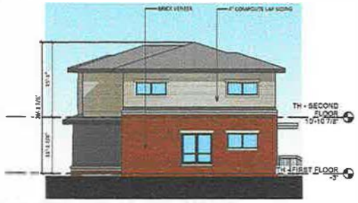
2 TH - SOUTH ELEVATION - COLOR 1/8" = 1'-0"
