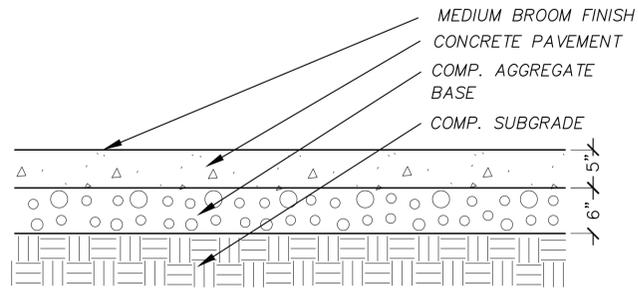
1 PED LOAD CONCRETE PAVEMENT-SECTION
