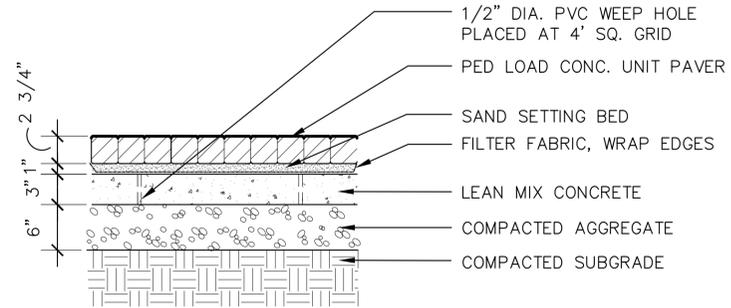
2 PED LOAD UNIT PAVER BAND - SECTION
