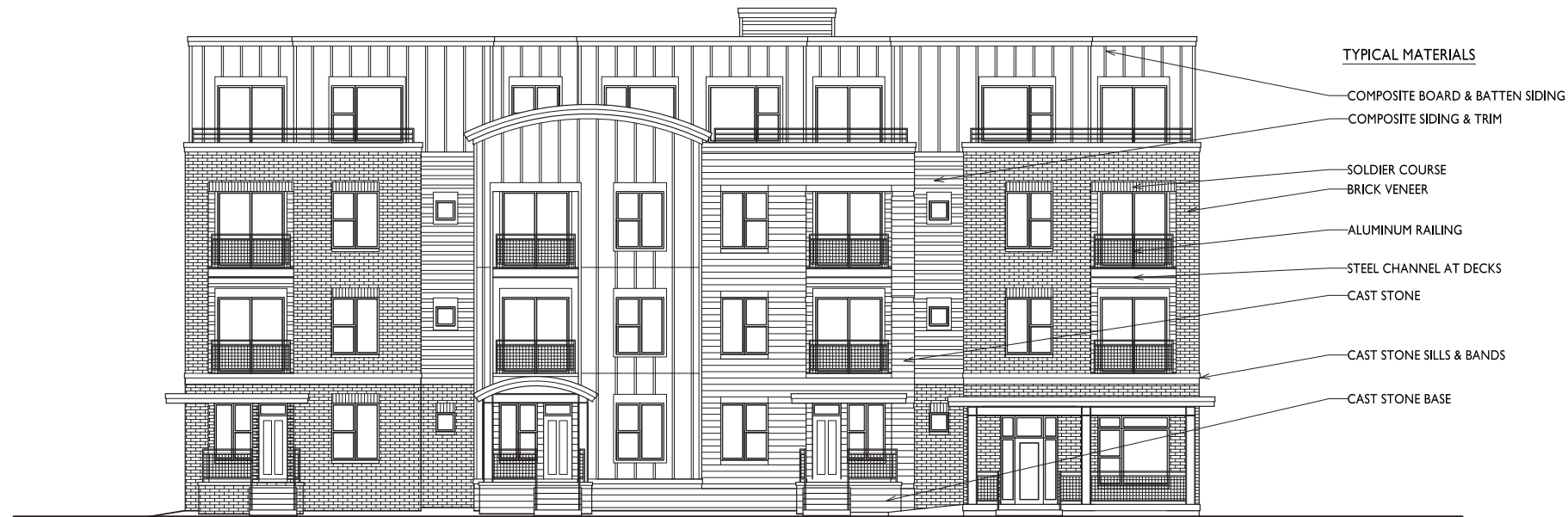
1 MIFFLIN ST. ELEVATION A-2.1 1/8"=1'-0"
