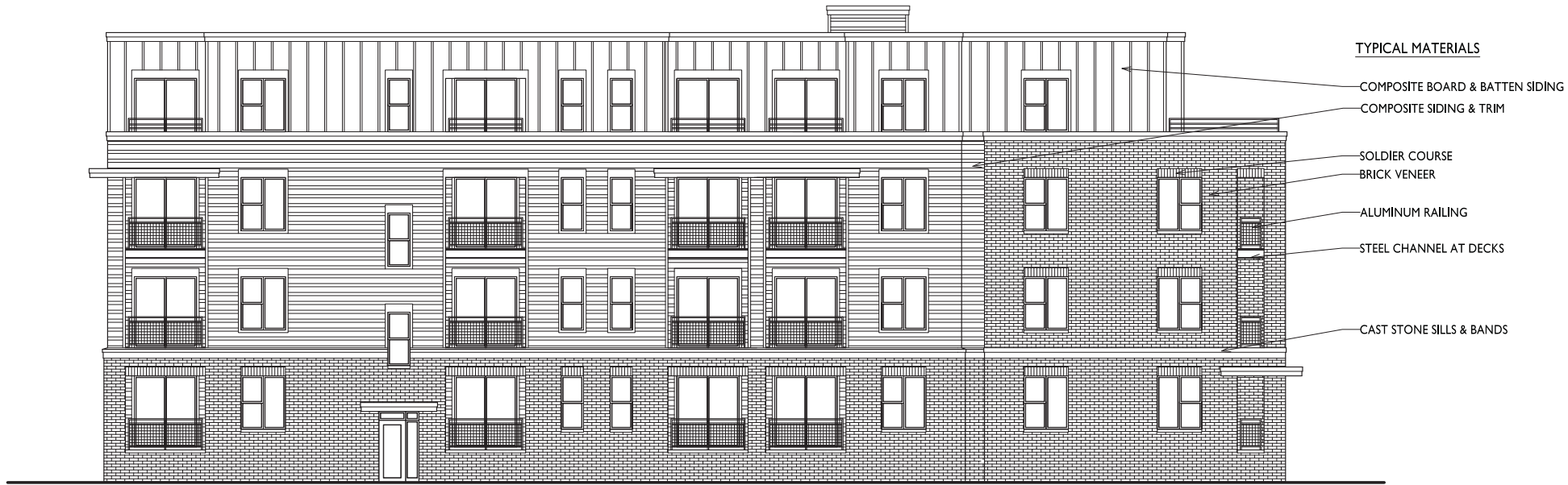
1 SOUTHEAST ELEVATION A-2.2 1/8"=1'-0"
