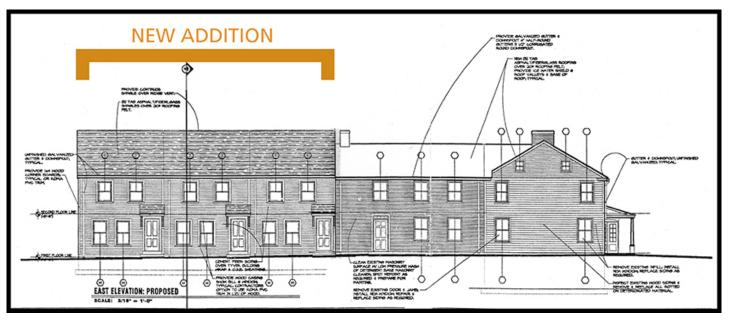
Figure 16. The proposal to add three row houses to the rear ell of this early-19th century residential property doubles its size and does not meet the Standards.
