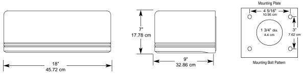
Note: Mounting plate center is located in the center of the luminaire width and 3.5" above the luminaire bottom (lens down position). Splices must be made in the J-box (by others). Mounting plate must be secured by max. 5/16" diameter bolts (by others) structurally to the wall.
