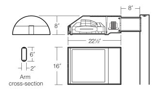
**Housing:** One-piece die-cast, low copper (<0.6% Cu) aluminum alloy with integral cooling ribs over the optical chamber and electrical compartment. Solid barrier wall separates optical and electrical compartments. Double-thick wall with gussets on the support-arm mounting end. Housing forms a half cylinder with 55° front face plane providing a recess to allow a flush single-latch detail. All hardware is stainless steel or electro-zinc plated steel.
