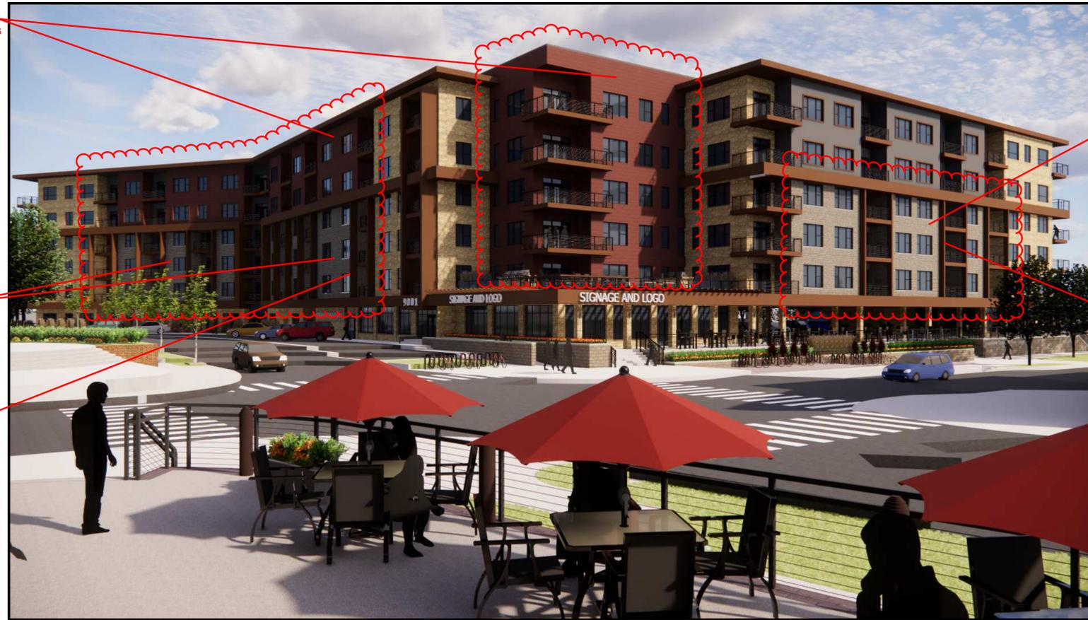
GRAY UTILITY BRICK REPLACED WITH SIMULATED WOOD PANEL. FACES OF WOOD PANEL WRAPS AND WOOD PANEL INFILL ARE NOW IN THE SAME PLANE.
