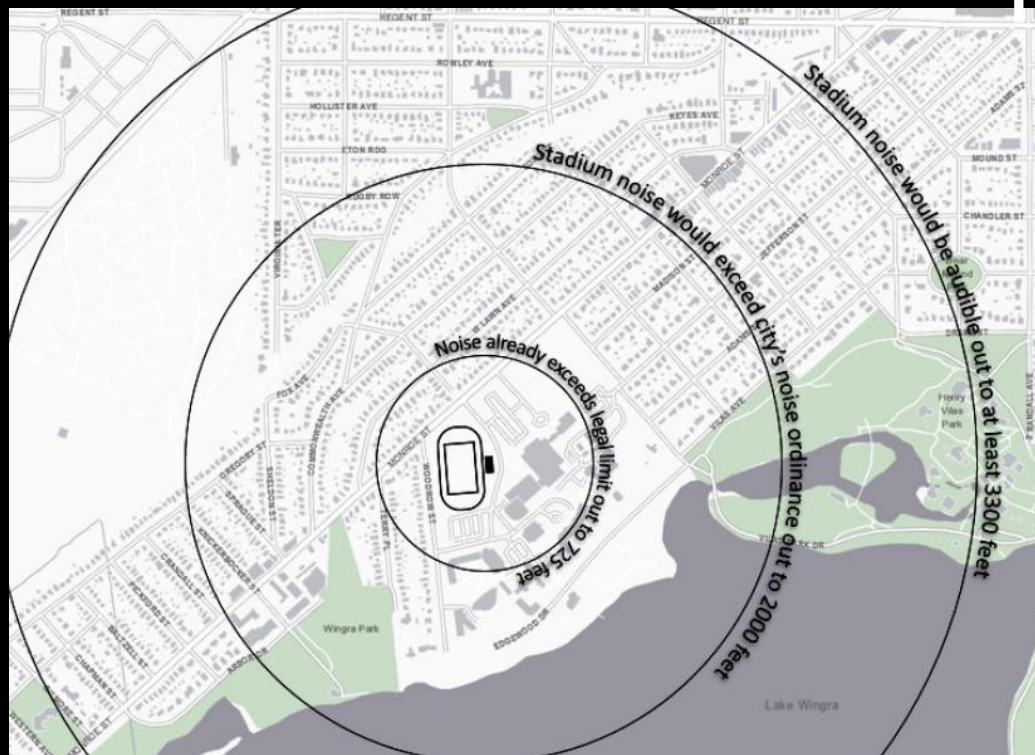
Figure 7 - Noise Model with Noise Barrier Shown
