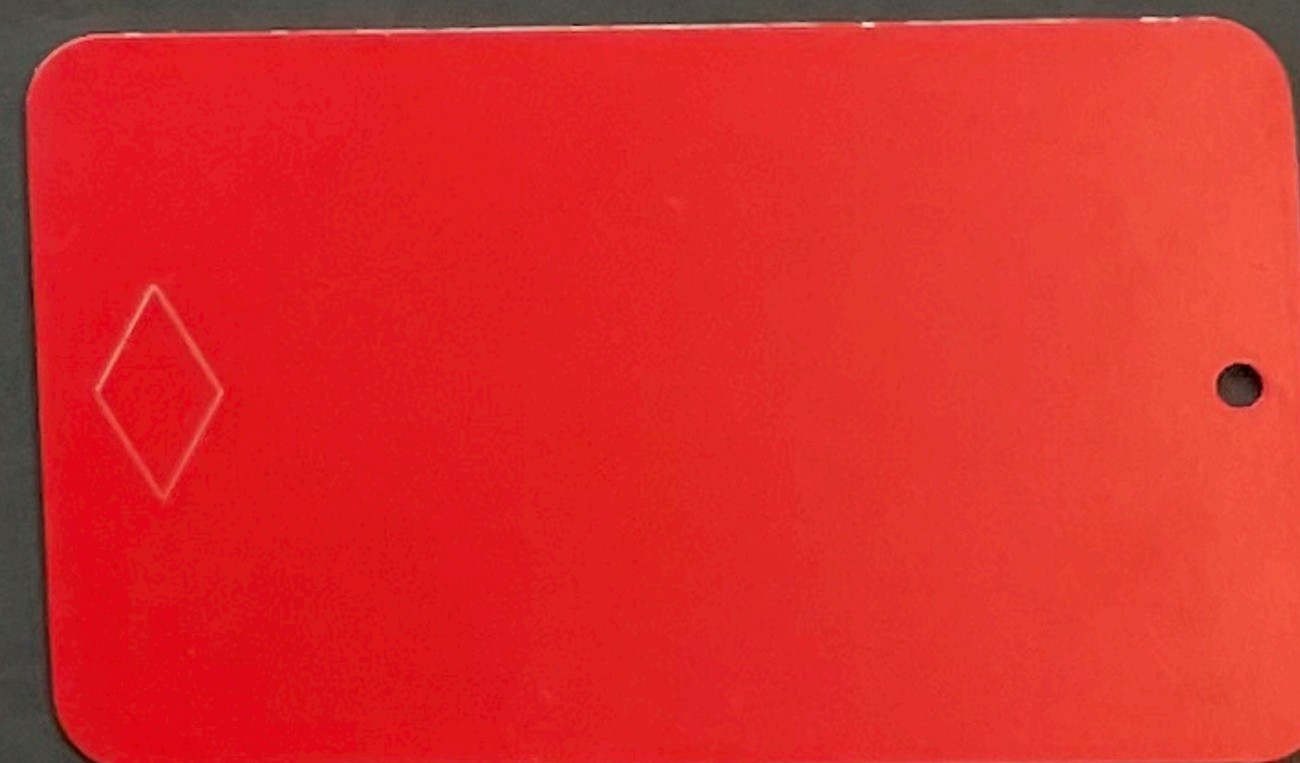
Flush aluminum ACM panels painted bright red
