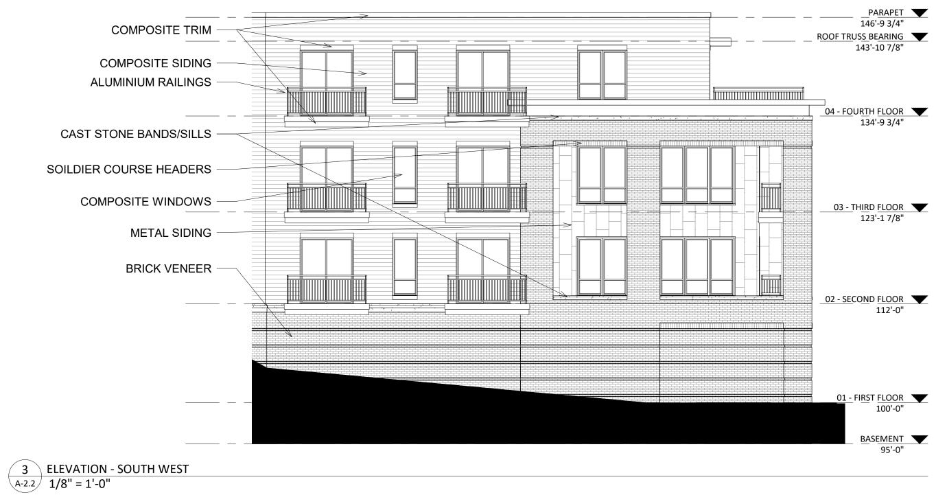
PARAPET \ 146'-9 3/4" COMPOSITE TRIM -ROOF TRUSS BEARING 143'-10 7/8" COMPOSITE SIDING **ALUMINIUM RAILINGS** 04 - FOURTH FLOOR 134'-9 3/4" CAST STONE BANDS/SILLS SOILDIER COURSE HEADERS COMPOSITE WINDOWS 03 - THIRD FLOOR 123'-1 7/8" METAL SIDING BRICK VENEER 02 - SECOND FLOOR 112'-0" BASEMENT 95'-0" 2 ELEVATION - SOUTH EAST A-2.2 1/8" = 1'-0"
