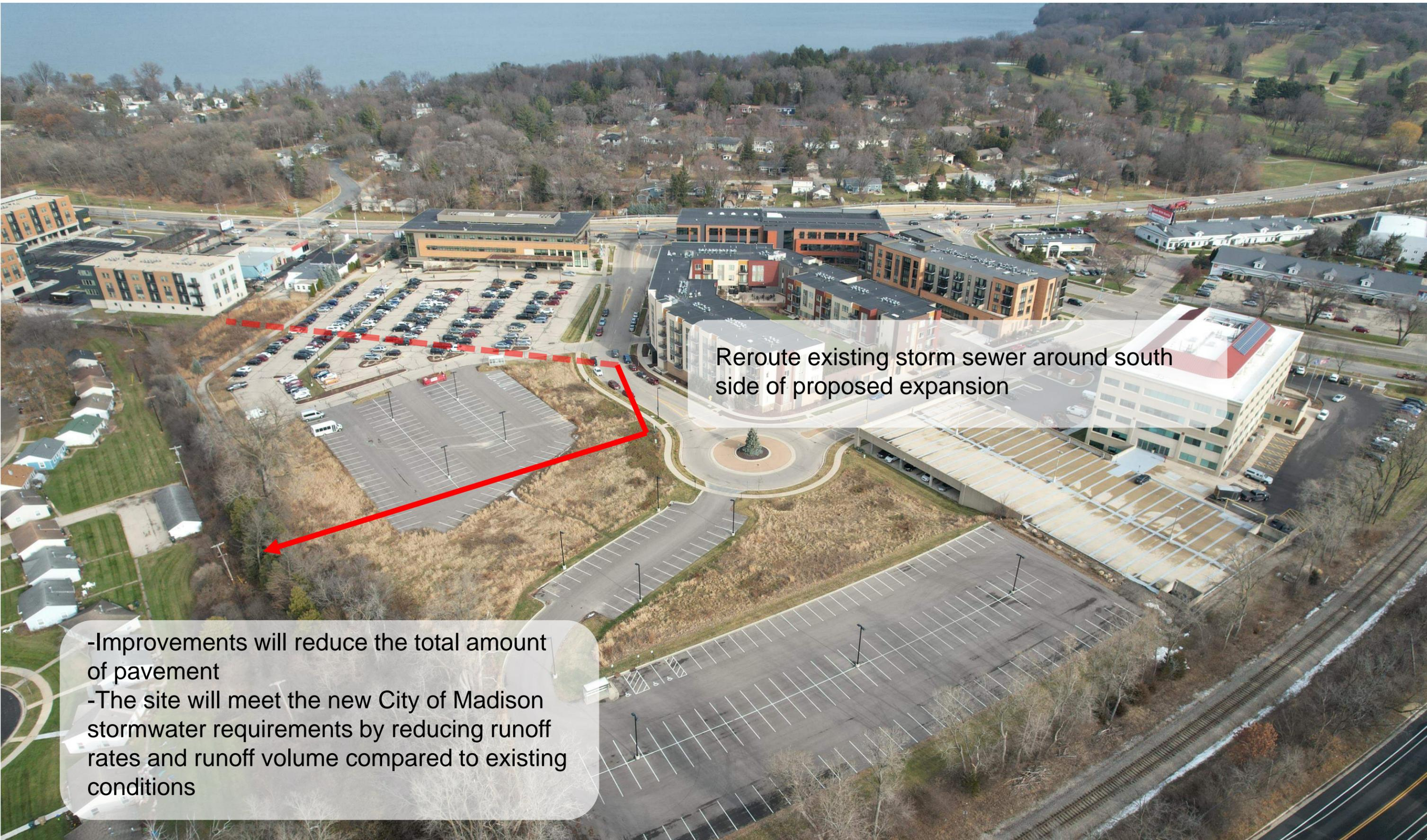
Reroute existing storm sewer around south side of proposed expansion
