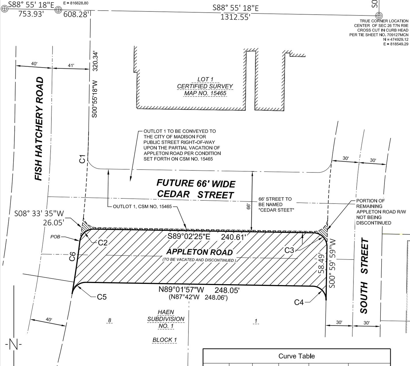
Bearings are referenced to the South line of the Northwest 1/4 of Section 26, which bears S 88°55'18" E on the Wisconsin County Coordinate System, Dane Zone NAD83(11)
