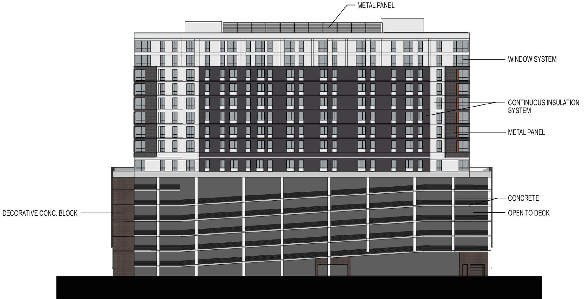
NOTE: ELEVATIONS ARE CONCEPTUAL AND SITE SURVEY AND ELEVATIONS NEED TO BE VERIFIED.
