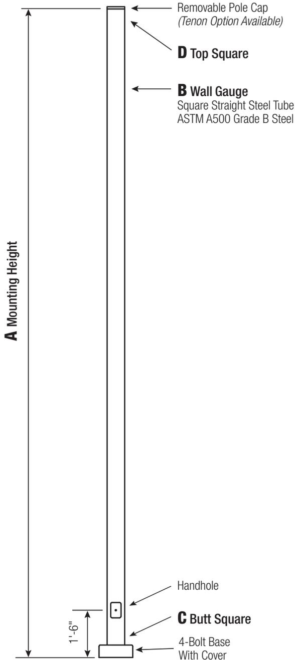
Powder Coated, Galvanized or Powder Coated over Galvanized Finish Per Customer Specification.
