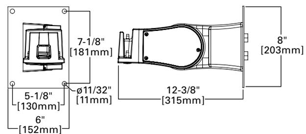
Adjustable Slipfitter (PRV & PRV-P)
