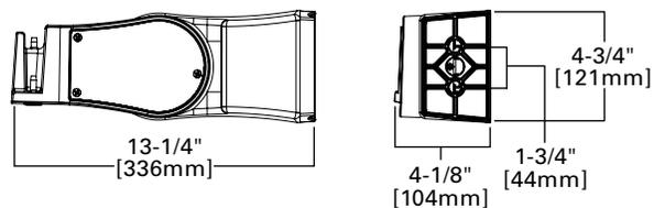
Adjustable Wall Mount (PRV & PRV-P)
