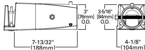
Adjustable Pole Mount Arm (PRV & PRV-P)
