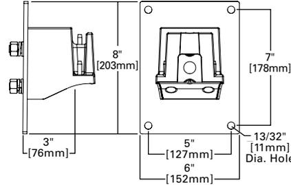
Mast Arm Mount (PRV & PRV-P)
